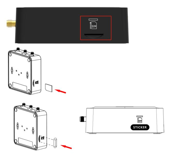
Insert or remove the SIM card as shown in the following steps.
