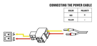
R1510 Router supports reverse polarity protection, but always refers to the figure above to connect the power adapter correctly. There are two cables associated with the power adapter. Following to the color of the head, connect the cable marked red to the positive pole through a terminal block, and connect the yellow one to the negative in the same way.
